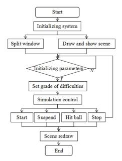
Fig. 4. Flow chart for system of simulation platform
